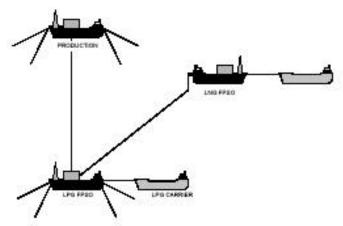
Eventually, the oil production FPSO and the LPG FPSO can be an integrated unit. Alternatively the LPG and LNG FPSO can be integrated into one vessel. It should be noted that the products including crude oil, LPG and LNG should be offloaded from the individual FPSOs to separate product carriers.
